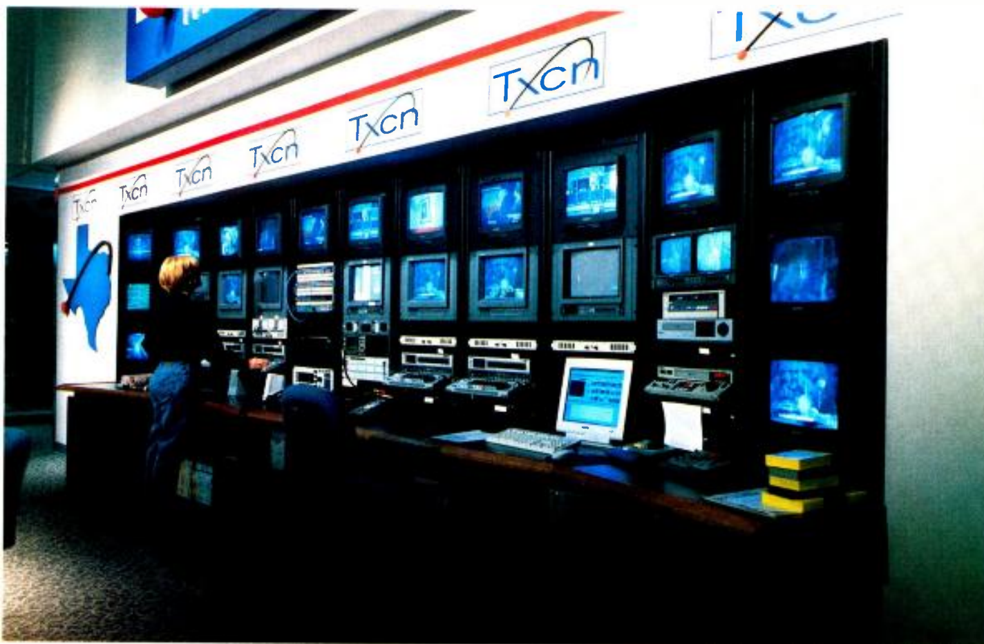
Nonlinear editing capabilities at Texas Cable News, Dallas, include Sony DNE-1000 editors networked to a central server system. This kind of arrangement allows non-technical staff to edit the news content they are producing. Photo courtesy Concept: Benson & Rice.
