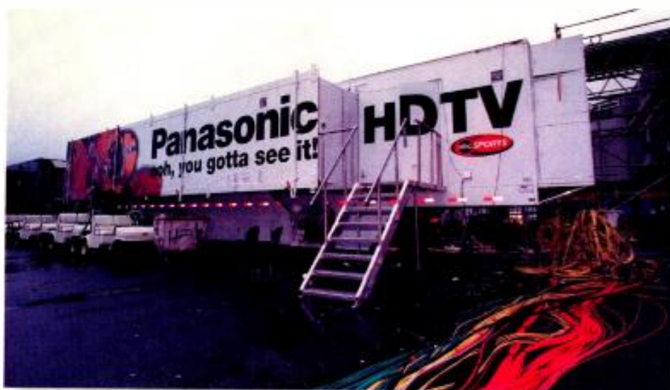
Mohawk/CDT fiber optic cable carried camera images from the field and broadcast booth to the truck. An additional camera feed was carried from the Coca-Cola Building via a Lucent Technologies Laser Link.
